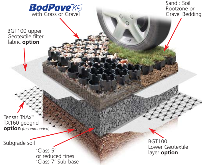
Integral interlocking 'snap-fit' connections on 19.7" x 19.7" grids
